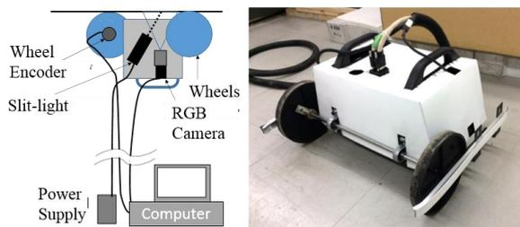
Figure 3. Mobile light-section device prototype
