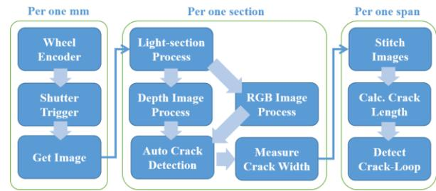
Figure 4. Crack inspection flow by the device
