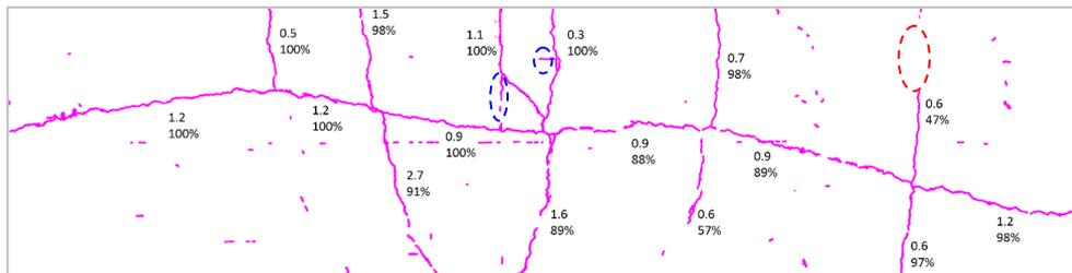
Figure 12. Auto crack detection result with crack width and crack detection rate
