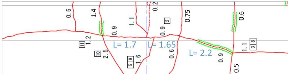
Figure 11. Inspection result by conventional method by inspection experts
