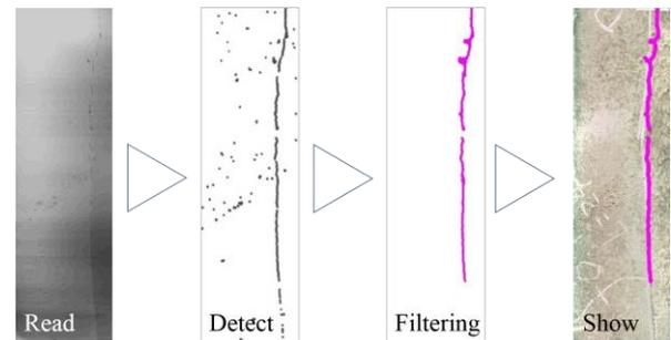
Figure 5. Flowchart of automatic crack detection
