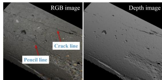
Figure 2. Tunnel inspection test by using our light-section device prototype
