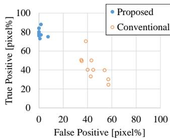
Figure 7. Automatic Crack detection accuracy by using 10 concrete test samples
