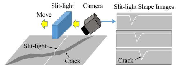
Figure 1. Concept of crack light-section device
