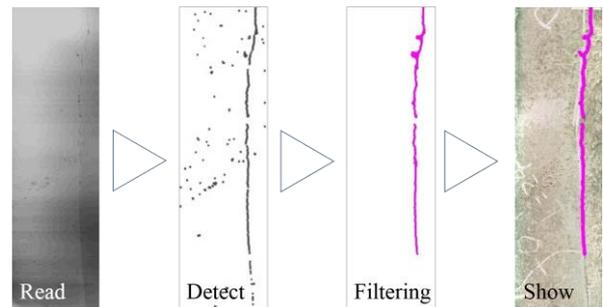
Figure 5. Flowchart of automatic crack detection
