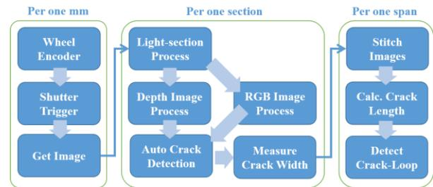
Figure 4. Crack inspection flow by the device
