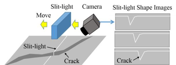
Figure 1. Concept of crack light-section device
