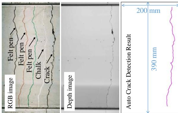
Figure 6. Automatic crack detection result example by using a concrete test sample with simulated dirt lines and a chalk line
