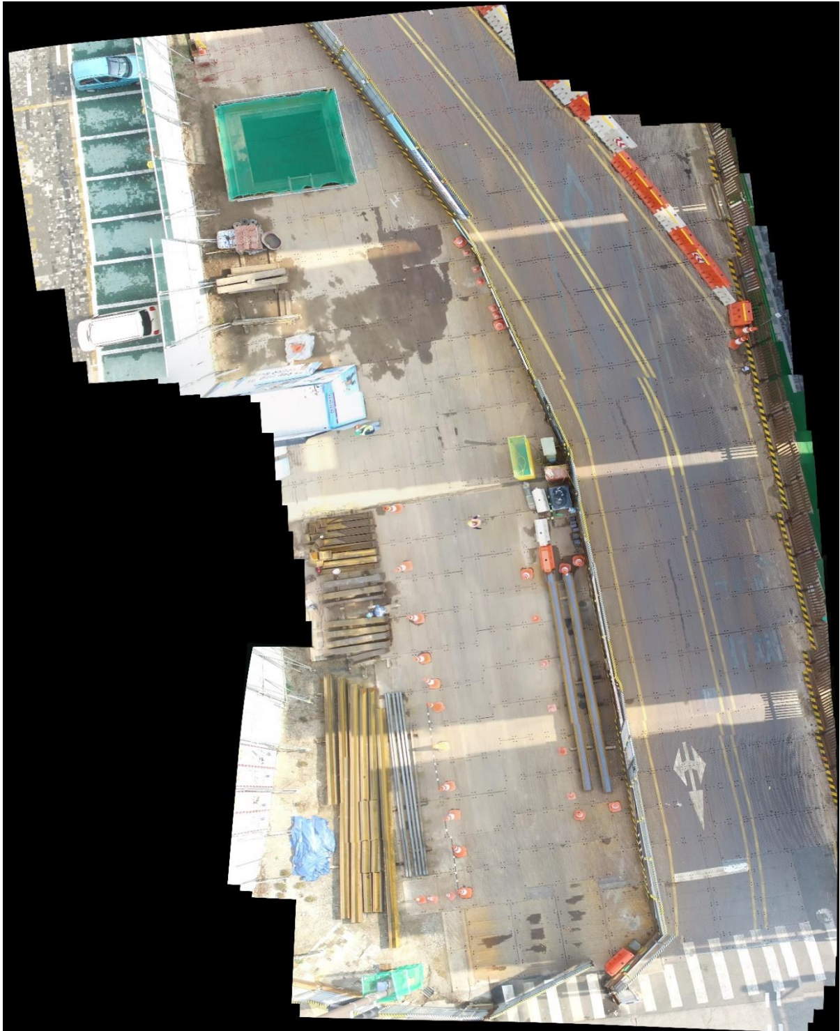
Figure 2. The result of 2D high-resolution map using the UAV video of the road construction site
