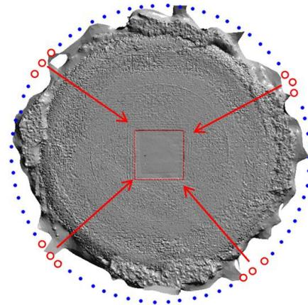
Figure.7 Camera positions for the twelve photographs selected given the six control points
