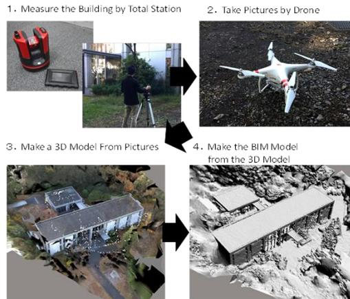
Figure.1 Typical procedure of UAV photogrammetry
