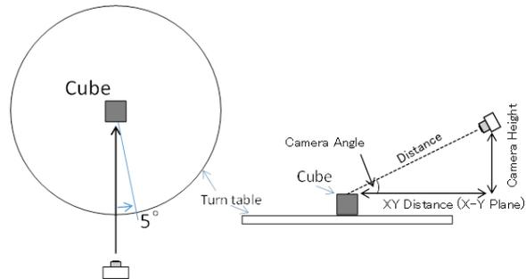
Figure.4 Positions of the camera and cube used in this experiment
