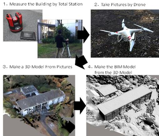
Figure.1 Typical procedure of UAV photogrammetry
