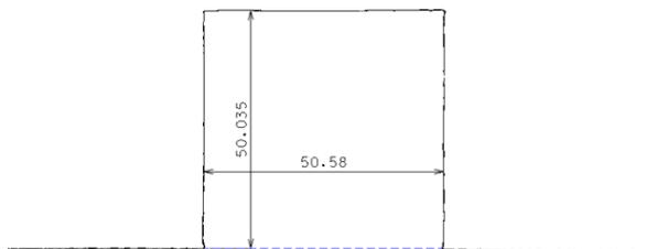
Figure.12 Cube dimensions in the X-Z plane
