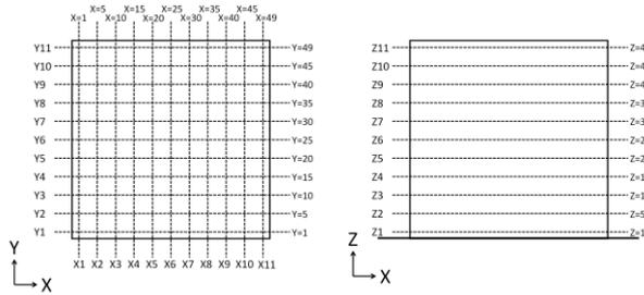
Figure.15 Measurement positions of the height and width dimensions
