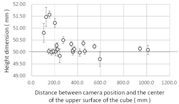
Figure.20 Relationship between the camera distance and the measurement accuracy
