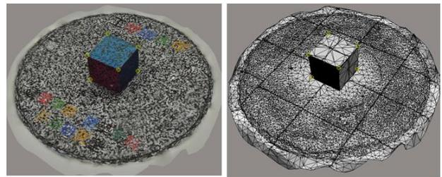
Figure.9 Example of a 3D model created from the photographs
