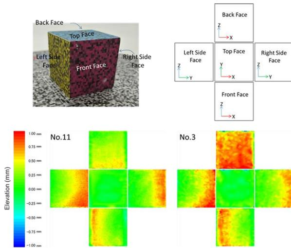
Figure.17 Accuracy of the measurement data for cube No. 3 and No. 11
