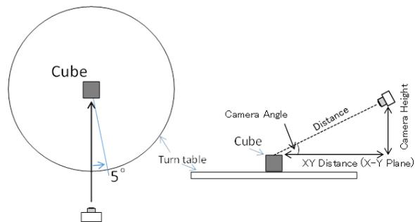
Figure.4 Positions of the camera and cube used in this experiment
