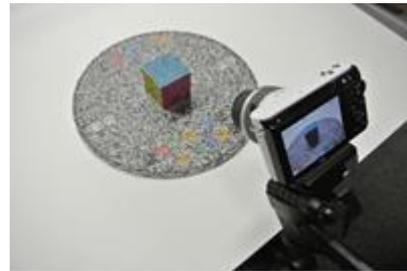
Figure.3 Camera setup in front of a cube on a turntable
