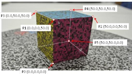
Figure.6 Six control points in this experiment
