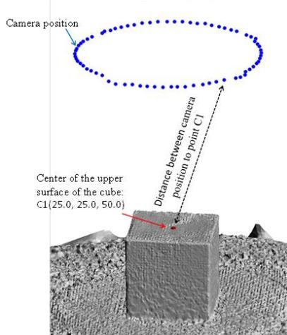
Figure.11 3D model and camera positions in 3D-CAD
