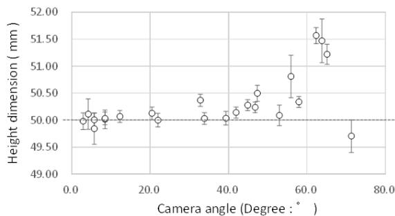
Figure.19 Relationship between the camera angle and the measurement accuracy
