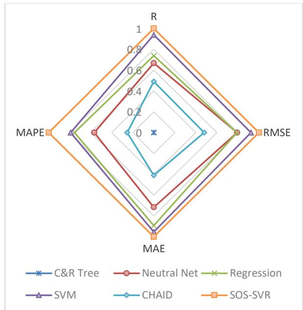
Figure 3. Radar plot of normalized accuracy measures (14-day strength test result)
