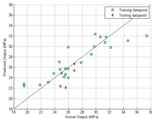
Figure 4. Actual and predicted concrete strength by SOS-SVR prediction model at training and testing stages for one fold (7-day strength test result).
