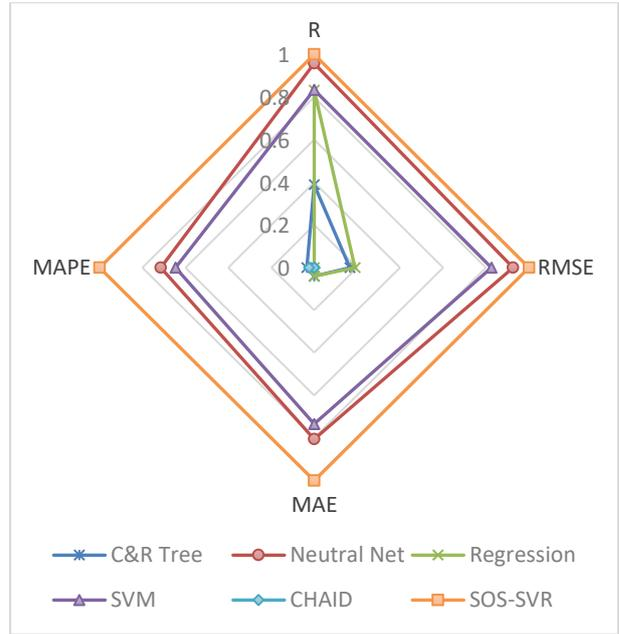
Figure 2. Radar plot of normalized accuracy measures (7-day strength test result)
