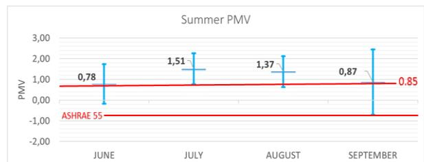
Figure 7. Thermal comfort during the summer and comparison with ASHRAE thresholds.
