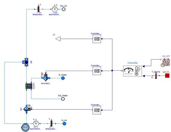
Figure 4. The sub-model of the fan coil.
