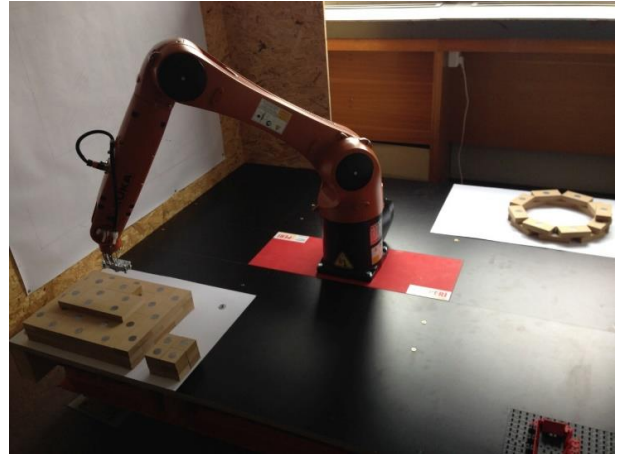
Figure 5 – De-palletizing by the robot (two pallet types – on the left)
