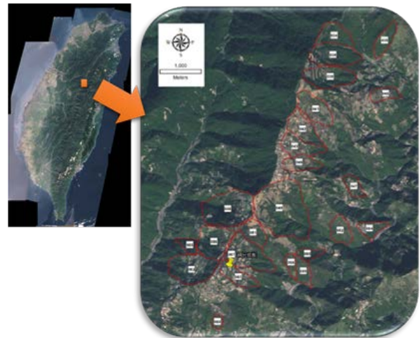
Figure 1 Landslide mapping with LiDAR data in study area.
