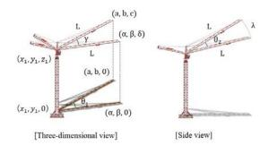
Fig 6. Images of tower crane displayed on threedimensional coordinate systems
