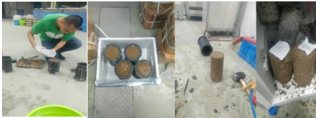
Figure 2. Preparation of frozen soil specimen
