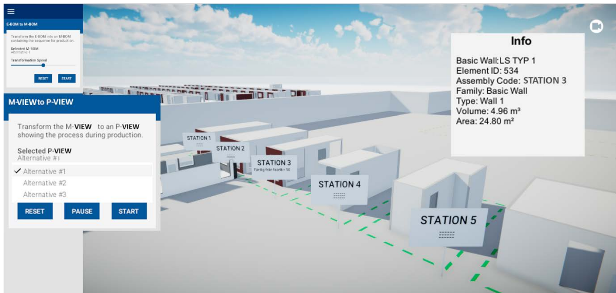
Figure 3. Visualisation of an alternative dialog and showing BIM information output with station related information in the factory production view in the IVE prototype
