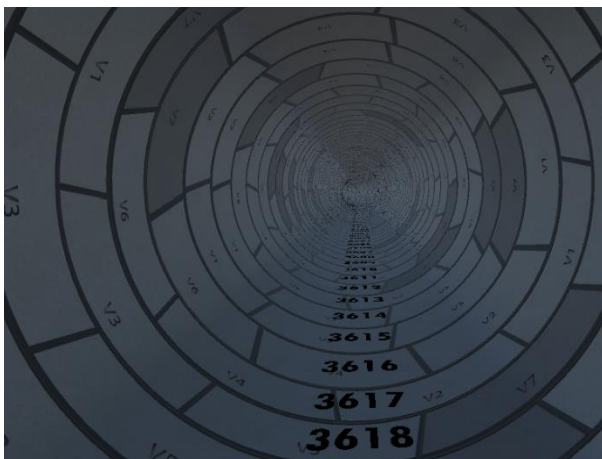
Figure 8: Semi-as-built tunnel model
