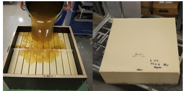
Figure 3. Grouting of cold wax tablets with hot wax to wax blocks (left) Cooled off wax block (right)
