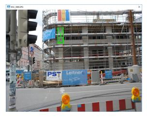
Figure 5. Reprojected triangulated column into a corresponding picture
