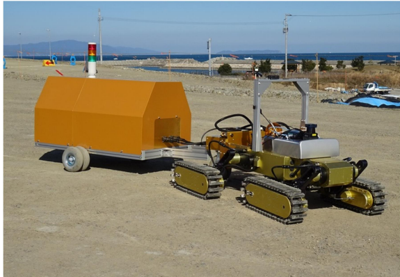
Fig. 5 Mobile robot and developed towing truck
