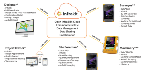
Figure 3. Automation system and operation models (Novatron Oy).
