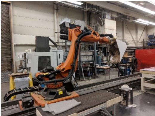
Figure 6. The simulated excavator by a robot arm mounted with an excavator bucket.
