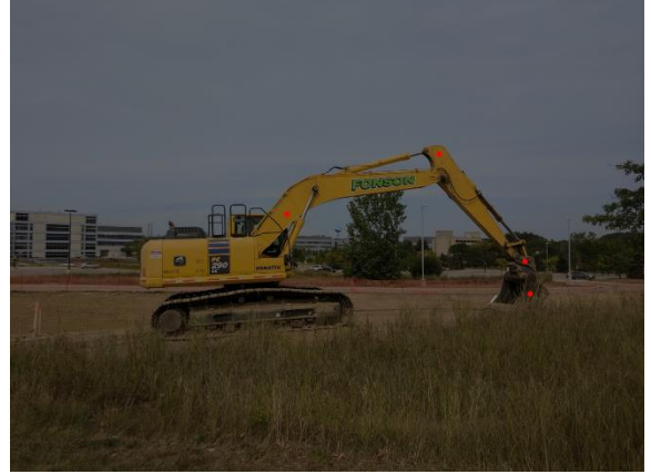
Figure 5. The concept of the prediction heat map. Each red dot represents the highest probability of each joint location.
