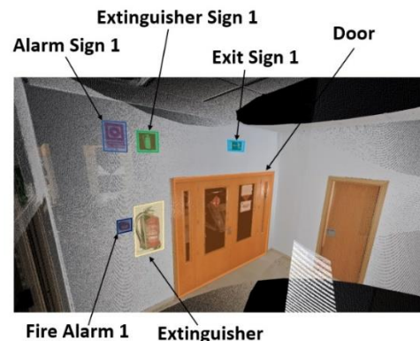
Figure 1. The image represents a coloured point cloud and different objects recognized in a wall. Apart from the doors, our recognition algorithm identifies five service building components.
