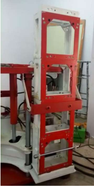
Figure 2. Modular column assembly by automation process: bottom to top assembly
