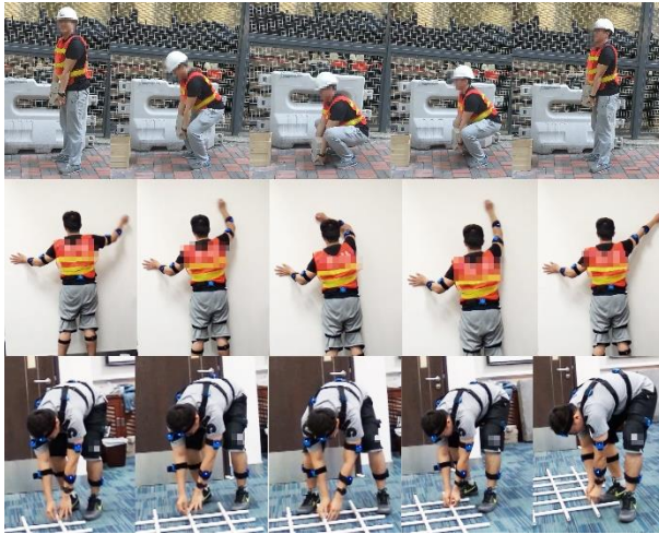
Figure 4. The example frames during material handling, plastering and rebar
