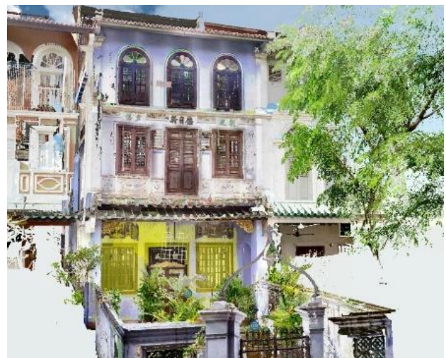
Figure 1. Sample point clouds of shophouse obtained from terrestrial laser scanning
