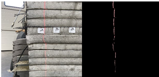
Figure 7: Manual laser line projection (left: RGB information, right: surface profile)
