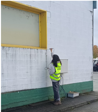
Figure 6. Reference temperature sampling using a Testo 720 probe.
