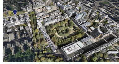
Figure 1. UAV-derived photogrammetric reconstruction of the University of Edinburgh Central Campus.
