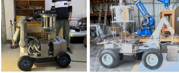
Figure 5. Experimental mobile 3D printing platform. Left: initial prototype with material hopper and extrusion system. Right: integrated system with 6-DOF robotic arm for terrain-adaptive printing.
