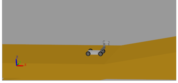
Figure 3. Simulink simulation environment showing the mobile robot traversing a slope terrain. The trajectory includes a 5-meter flat section followed by a 5-meter slope at 5^\circ inclination.
