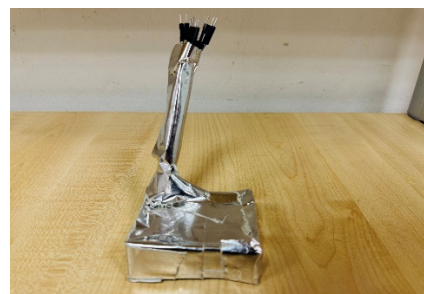
Figure 6. Sealed control electronics enclosure for underwater operation
