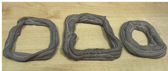
Figure 5. Printed cement specimen
