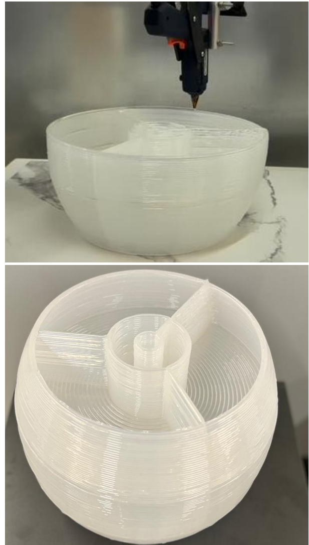
Figure 6. 3D Printed Scaled Model of the Marsphere
