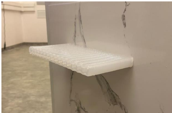
Figure 7. 3D printed cantilever slab
