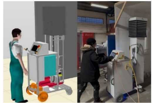
Figure 4. Digital twin (left) of real robot-based spraying process (right) within the simulation software ema Work Designer.
