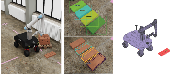
Figure 5. Mobile robot setup in Isaac Sim (left) publishing RGB-D image data for the real-time brick pose estimation (middle), and registration of the estimated poses in the modelling environment (right).
