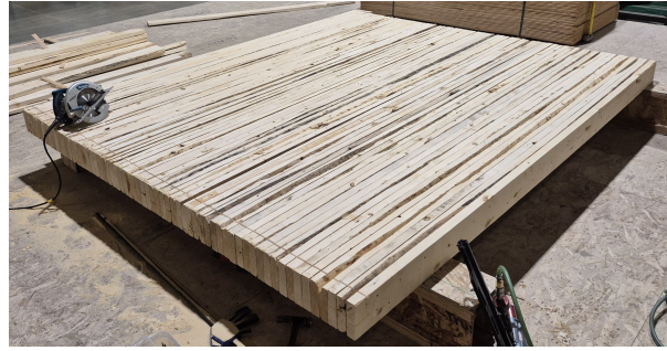
Figure 7. Manually fabricated NLT panel after completion of the full assembly process.
