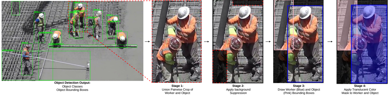
Figure 2. The preprocessing stages applied to each candidate pair in both deployment strategies. The red dotted outline is shown for illustrative purposes only and is not part of the candidate crop.
