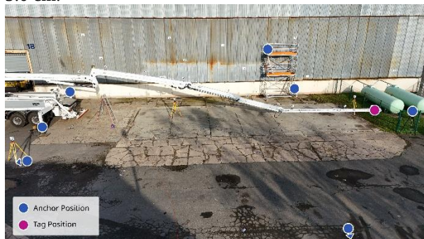
Figure 5. Positions of the anchors and the tag around the concrete pump used in the experiment
