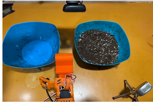
Figure 2. Experimental setup showing the robotic arm, bowls, and multi-camera configuration for data capture.
