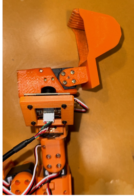
Figure 1. Modified SO-101 robotic arm with 3D-printed excavation bucket.
