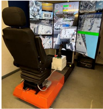
Figure 1: Remote-controlled tower crane cabin
