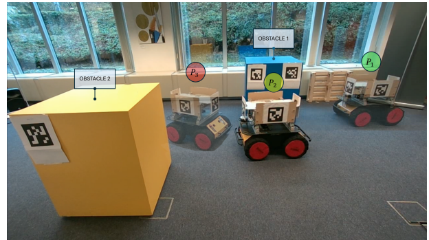
Figure 1. Mobile robot avoiding obstacles. The initial position is denoted by P_1 . While P_2 , and P_3 are intermediate locations toward reaching the goal.
