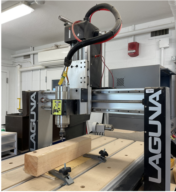
Figure 6. The clamping setup of the joint with the Laguna CNC [18].
