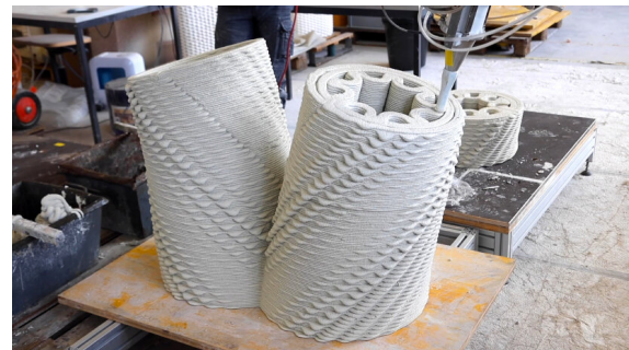
Figure 9. Case 3 - Tor Alva - off-site 3D Concrete Printing process by dbt [26].
