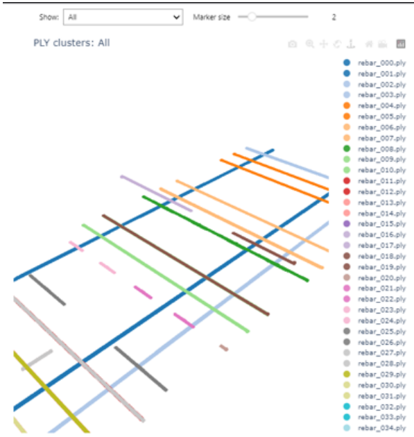
Figure 5. Segmentation results of using cylinder-model fitting
