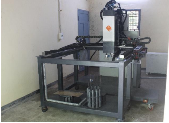
Figure 3 An early physical prototype of the baseline single-gantry design (ND) integrating 3D printing with robotic pick-and-place features.
