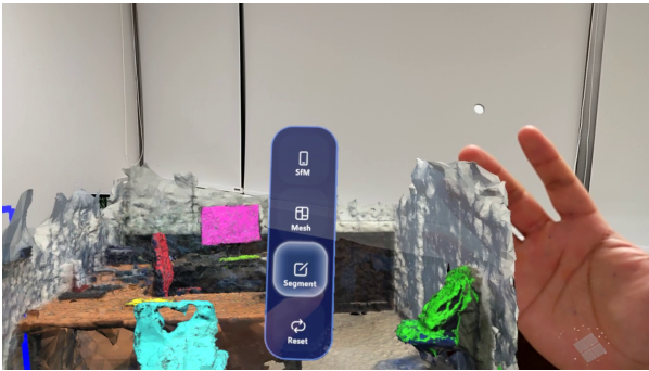
Figure 7. Semantically enriched 3D mesh visualized in the XR environment.
