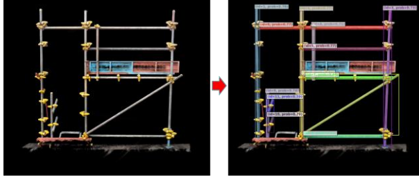
Figure 5. 3DGS-based structure decomposition and VLM-enabled component recognition. The left image shows the cropped frontal view of the scaffold's 3DGS model; the right image illustrates the segmentation results using the text prompt “bar”.
