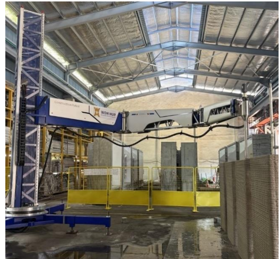
Figure 2: Printing of 3DCP walls
