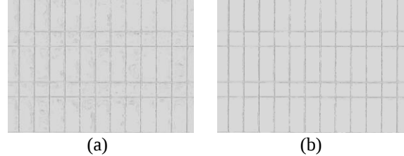
Fig. 6 Geometric correction by (a) simply overlapping and (b) cuboidal region replacement
