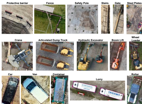
Figure 2: Labelled objects used for this work to monitor the construction site layout activity.
