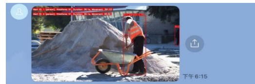
Figure 7. Example of hazard alert notification delivered via the LINE BOT interface.
