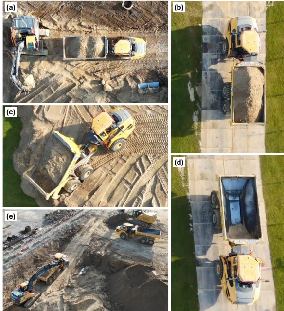
Figure 4. Observed dump truck duty cycle: (a) Load, (b) Haul, (c) Dump, (d) Return, and (e) Wait.
