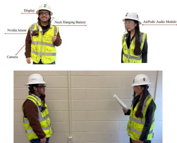
Figure 2. Wearable system configuration and physical implementation
