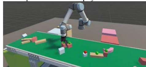
Figure 4. Unity based conveyor DT with dynamically spawned waste objects generated from RGB annotations. The environment includes the conveyor, simulated robot arm, and physics-based object interactions.
