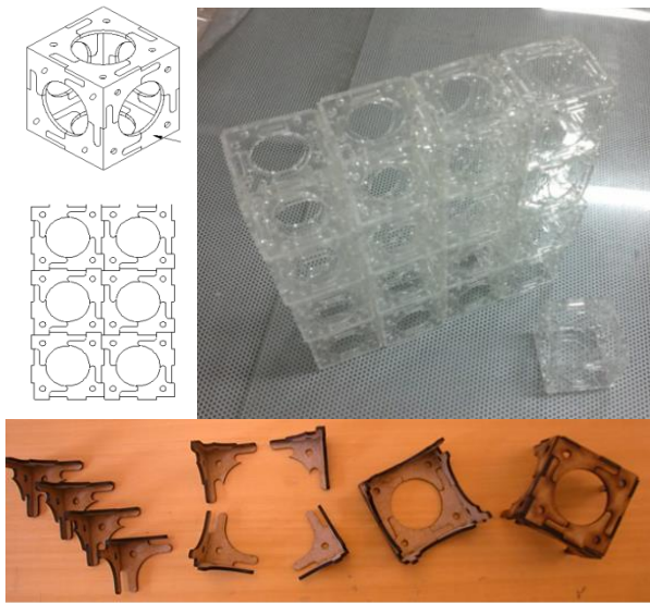
Figure 1. Component design with MDF (Laser cutter)
