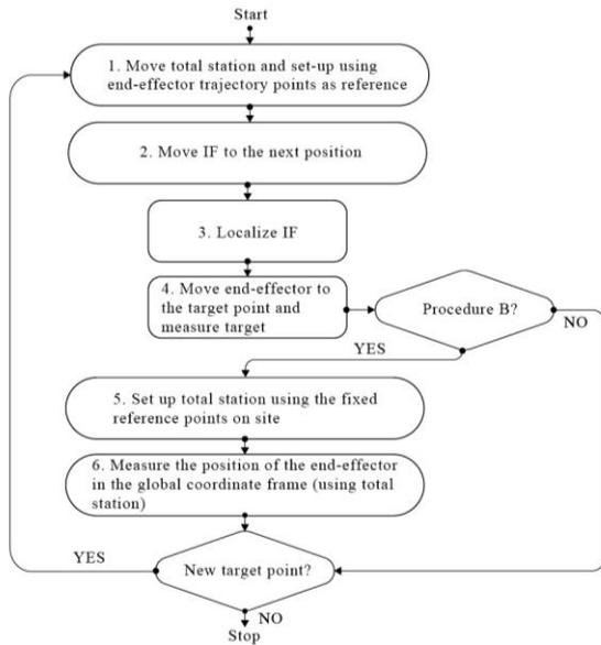
Figure 4. The full experiment flow for the acquisition of one data point.
