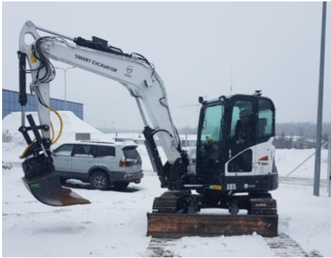
Figure 6. The University of Oulu's Smart Bobcat E85 Excavator.
