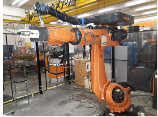
Figure 8. G2 sensor testing using a KUKA robot manipulator
